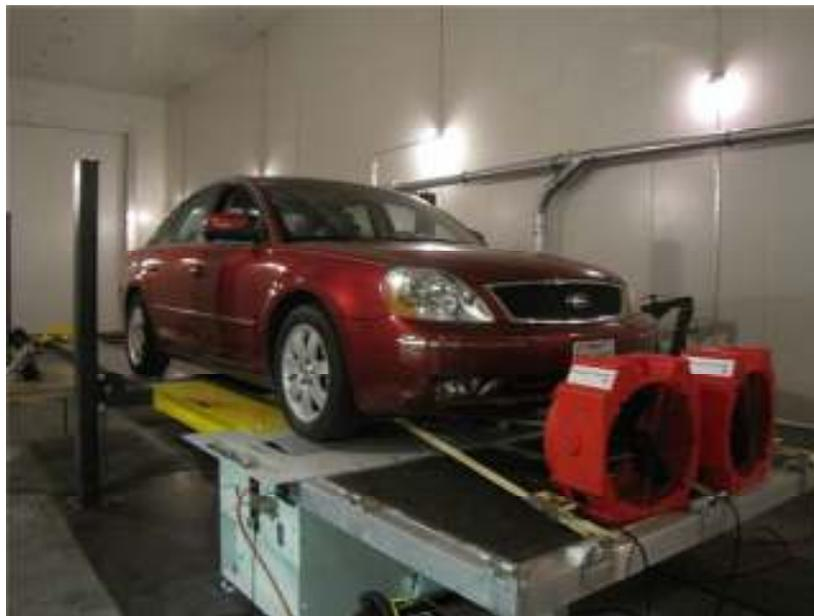
Figure 1: Test Vehicle on Dyno in Chamber
